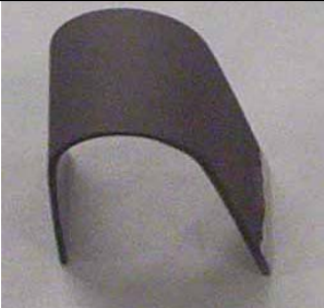
PComp™ coating bent 360 degrees, showing absence of cracking or spallation
